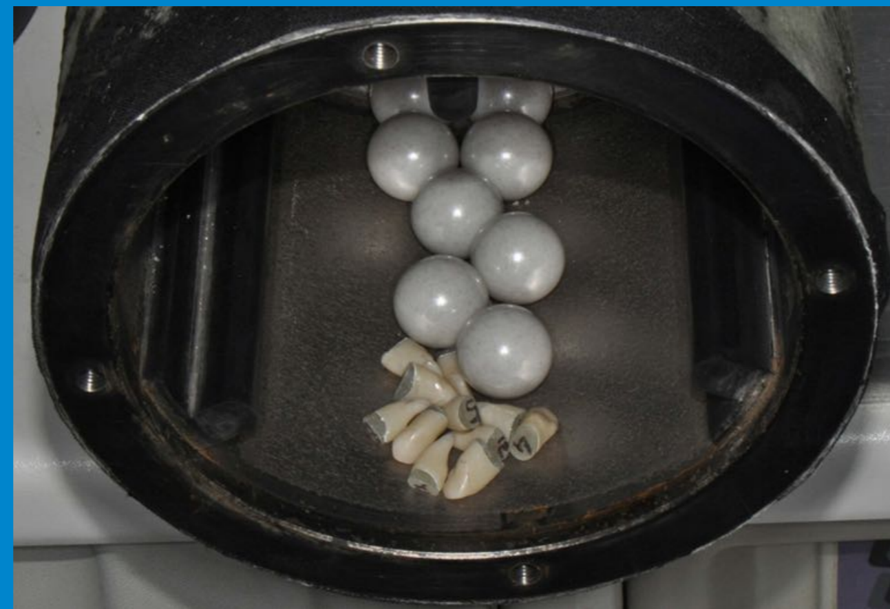
The Ball Mill fatigue machine: the drawing shows the kinetic of the spheres (zirconia ceramic) which generate damage accumulation on the ceramic restoration. from: Abu Kasim NH. The ball mill as a means of investigating the mechanical failure of dental materials. J Dent. 1996 Jan-Mar;24(1-2):117-24.
