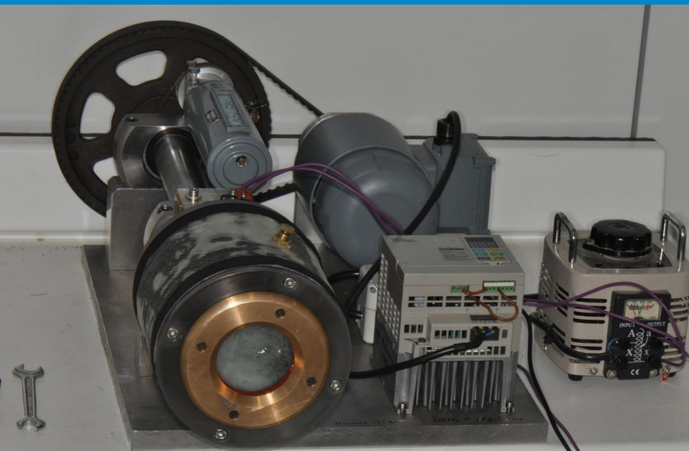
The Ball Mill fatigue machine: the drawing shows the kinetic of the spheres (zirconia ceramic) which generate damage accumulation on the ceramic restoration. from: Abu Kasim NH. The ball mill as a means of investigating the mechanical failure of dental materials. J Dent. 1996 Jan-Mar;24(1-2):117-24.
